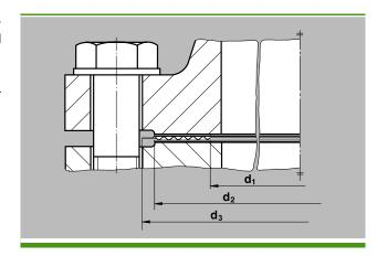
Works standard 210 For smooth flanges and flanges with raised face as per DIN and/or EN
