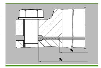
Conforms to EN 12560-4 for flanges in accordance with ANSI B 16.5
