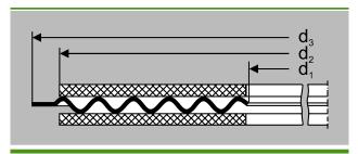
As the external diameter of the layers is approx. 8 mm smaller than the corrugated carrier, this identification area is always visible.
